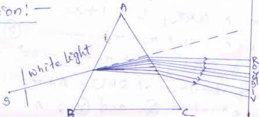
Dispersion is the phenomenon of light by virtue of which a white light passing through a prism and splits up into its constituent colours.
