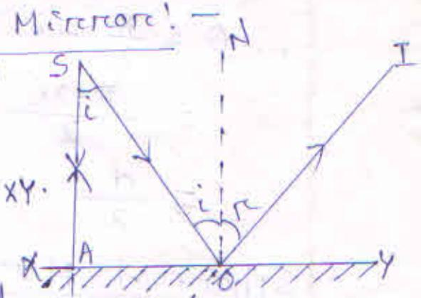
Conclusion: — The image formed at the same distance behind the mirror. It is virtual of same size and laterally inverted.
