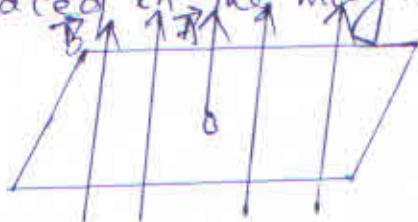
Magnetic field linked with a surface is maximum when area is held perpendicular to the direction of magnetic field.
