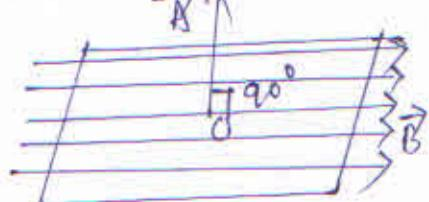
No magnetic flux is linked with the surface when the field is parallel to the surface.
